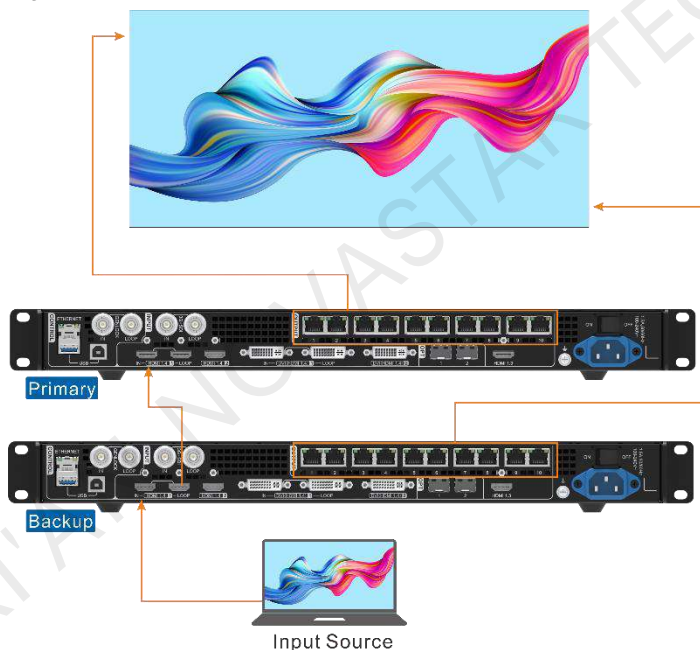
Figure 5-25 Device backup connection
